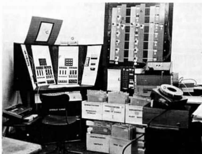
Fig. 1.1. The INTUITION System. Typical working station. A = Entailment structure display (probability theory). B = Node with state marker lamps, sockets, contacts, labels; used in transactions described in the text. C = Screen for display of descriptor examples and counterexamples through random access projector. D = Random access projector. E = Check list device. F = Modelling facility for subject matter or probabilistic theory, STATLAB. G = "Boxes" used for conditional probability experiments. H = Tape recorder for inputting random or quasi random "natural results" together with spoken commentary on the external demonstration. I = Files containing "layover cards" for STATLAB, other demonstration material and aim validation cards for insertion in mini BOSS (not shown in this photograph). J = Control and recording mechanism which may be interfaced with minicomputer for class (not shown in this photograph). K = Student position.
