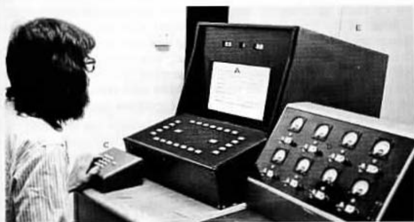
Fig. 1.5. Arrangements used in semi-mechanised free-learning and teachback experiments on learning style. A = Back projection unit for displaying examples. B = Selection buttons and signal lamps. C = Auxiliary indexing buttons. D = Confidence estimation equipment for determining look ahead uncertainty or topic uncertainty as numerical values. E = Lower point of the entailment structure (facing student but just visible in photograph).
